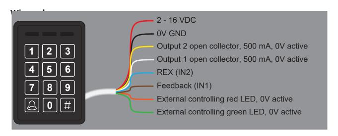
**Note:** Right after applying the voltage all LED's lights and the buzzer sounds **do not** touch the reader untill the yellow LED lights and the buzzer is silent.
