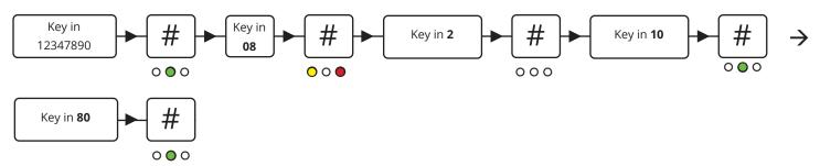
When the battery is running low it will give you a warning when you type in your user code. The red LED will flash while the buzzer beeps for about 3 seconds. The output is hereafter activated.
