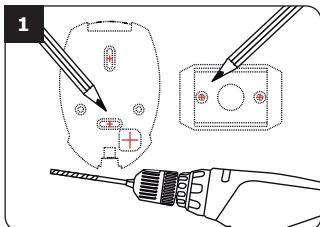
Verify the distance between the GALEO keypad and its remote electronic (Refer to page 3 «Notes and Recommendations»). Place the back plate of the GALEO on the wall and the bracket of the remote electronic then mark with a pen the hole location then drill the 2 mounting holes (drill bit Ø 5 mm and 35 mm hole depth) and the hole wiring access.
