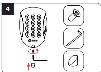
Fasten the GALEO keypad to the back plate by using the supplied (M4x10) Torx® screw and T20 Trox spanner hardware. Place the screw cap at the bottom of the keypad.
