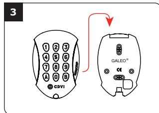
Insert the cable in the hole access area of the back plate. Then mount the keypad on the back plate, placing first the top in the hooks and then the bottom.
