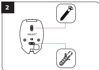
Insert the 2 plastic anchors in the holes. Place the back plate of the GALEO and screw on the wall using the supplied (M4x30) mounting screws.
