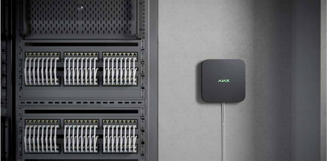
It is advisable to choose an installation site where NVR is hidden from prying eyes— For example, in the pantry. This will help reduce the likelihood of sabotage or jamming of the security system. Note that the device is intended for indoor installation only.
